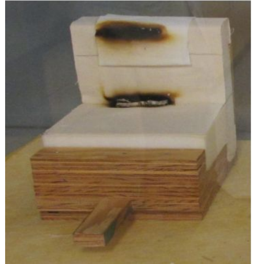
Example of TB 117-2013-style mockup posttest. Char length is measured up from the crevice vertically.
